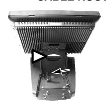
For cable routing in the mini slim base, please refer to the picture at left. There is a cable tie inside the base trunk as arrowed in the picture. Hold all the external cables with the cable tie. Have all cables to pass through the oval hole on the trunk as triangle marked to come out of the front side of trunk. Connect all the cable ends to main unit. Should there is the option SATA HDD in base installed, please double check that the HDD cables must be still secured.
